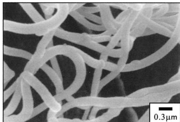
Figure 4 Fibril structure appeared on the fracture surface of annealed sample under impact loading.
